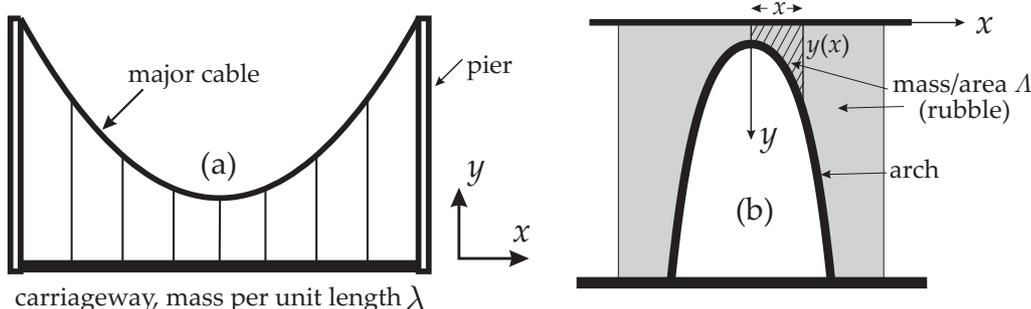
**Figure 9:** (a) A suspension bridge where the major cable supports a carriageway. (b) A Roman bridge in the form of a light arch supporting a rubble fill above it on which a carriageway sits.
